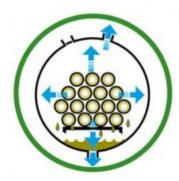
Final vacuum extracts excess preservative solution, which is pumped back to storage.
