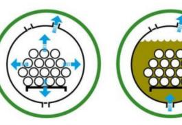
Timber loaded into treatment vessel. Initial vacuum applied and the timber cells are evacuated of air. Vacuum held.
