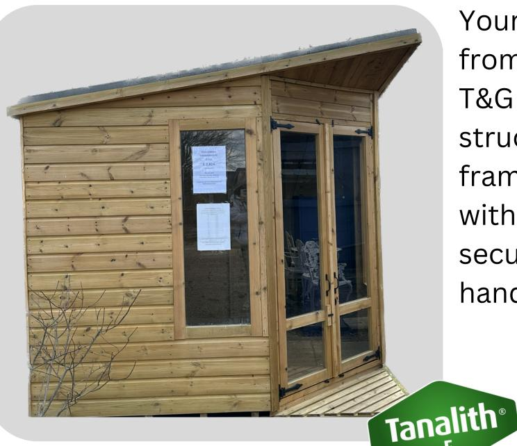
Your Summerhouse will be constructed from 16mm pressure treated tanalised T&G wood, to ensure a sturdy and robust structure with robust 3 x 2 (60 x 40mm) framing and toughened safety glass. Along with the addition of traditional and ornate secure hinges with lock and key, pull handles and a 3" turn buttons as standard.
