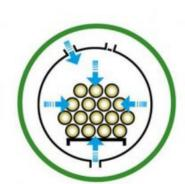
Low pressure inside timber draws in surface solution when vented to atmosphere. Treated timber is left to dry.
