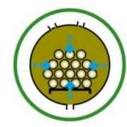
Hydraulic pressure applied, forcing the preservative deep into the structure of the timber.
